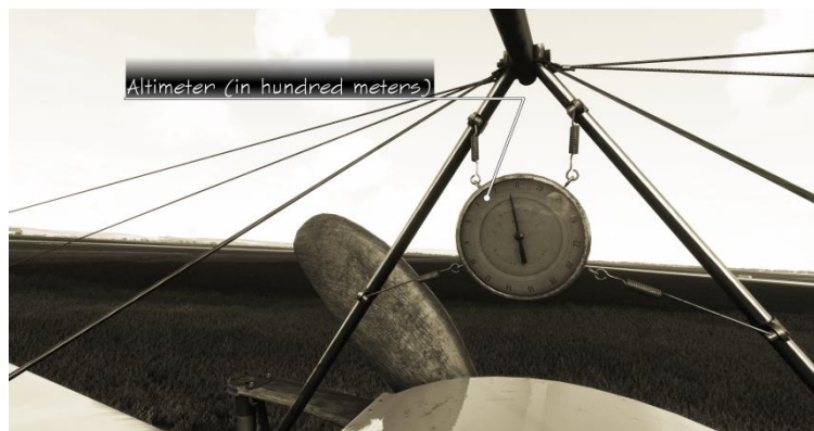
Figure 8: Modern Instrumentation: the Naudet altimeter.
