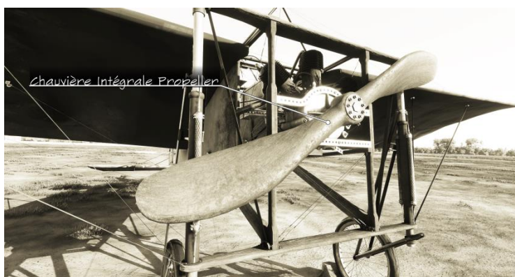
Figure 11: Front view of the aircraft. Pull the propeller to start the engine.
